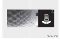
You can change Rear View Monitor 'Display Contents' or 'Display Settings' by touching the setup icon (♠) on the screen while the Rear View Monitor is operating, or selecting 'Driver Assistance → Parking Safety → Camera Settings' from the Settings menu while the engine is on.
