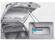
Your vehicle is equipped with the emergency tailgate safety release lever located on the bottom of the tailgate. When someone is inadvertently locked in the luggage compartment, the tailgate can be opened by doing as follows:
