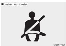
As a reminder to the driver, the driver's seat belt warning light will illuminate for approximately 6 seconds each time you turn the ignition switch or Engine Start/Stop button ON regardless of seat belt fastening.
