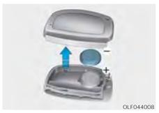
If the Smart Key is not working properly, try replacing the battery with a new one. Battery Type: CR2032
