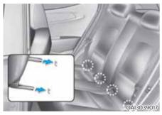
Both rear outboard seats are equipped with a pair of ISOFIX anchorages as well as a corresponding top-tether anchorage on the back side of the rear seats.
