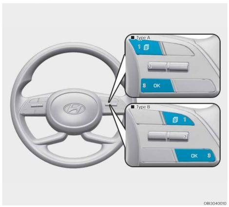
The cluster display modes can be changed by using the control buttons.
