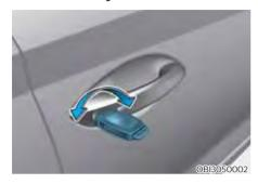
Turn the key toward the rear of the vehicle to unlock and toward the front of the vehicle to lock.
