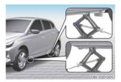
7. Place the jack at the designated jacking position under the frame closest to the tire you are changing. The jacking positions are plates welded to the frame with two tabs and a raised dot. Never jack any other position or part of the vehicle.
