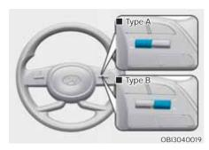
To change the trip mode, toggle the " \( \lambda \, \sup " \) switch on the steering wheel.
