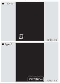
This indicator displays which intelligent variable transmission shift lever is selected.
