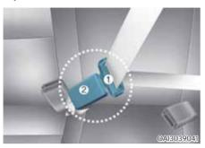
Insert the tongue plate (1) into the buckle (2) until an audible "click" is heard, indicating the latch is locked make sure the belt is not twisted. When using the rear center seat belt, the buckle with the "CENTER" mark must be used.
