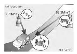
Multi-Path Cancellation - Radio signals being received from several directions can cause distortion or fluttering. This can be caused by a direct and reflected signal from the same station, or by signals from two stations with close frequencies. If this occurs, select another station until the condition has passed.
