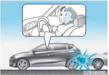
Front air bags are not designed to inflate in rear collisions, because occupants are moved backward by the force of the impact. In this case, inflated air bags would not be able to provide any additional benefit.
