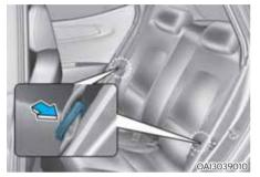
Insert the rear lap/shoulder belt plate into the holder on the side trim. It will prevent the lap/shoulder belt from interfering with the seatback when folding.
