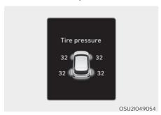
When the tire pressure monitoring system warning indicators are illuminated and a warning message displayed on the cluster LCD display, one or more of your tires is significantly under-inflated. The low tire pressure position telltale light will indicate which tire is significantly under-inflated by illuminating the corresponding position light.
