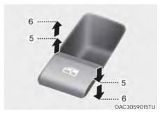
Pressing the power window switch momentarily to the second detent position (6) completely lowers the driver's window even when the switch is released. To stop the window at the desired position while the window is in operation, pull up and release the switch to the opposite direction of the window movement.
