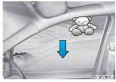
If a window senses any obstacle while it is closing automatically, it will stop and lower approximately 30 cm (12 inches) to allow the object to be cleared.
