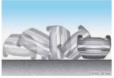
Air bags do not inflate in rollover accidents because the vehicle can not detect rollover accident.
