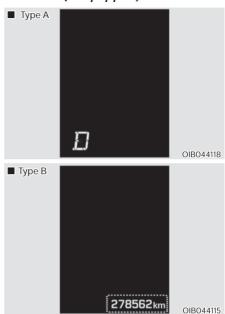
This indicator displays which dual clutch transmission shift lever is selected.
