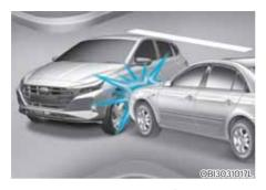
Front air bags may not inflate in side impact collisions, because occupants move to the direction of the collision, and thus in side impacts, frontal air bag deployment would not provide additional occupant protection.
