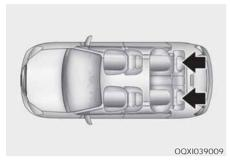
The rear seats are equipped with headrests in the outboard seating positions for the occupant's safety and comfort.
