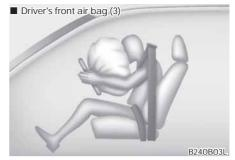
A fully inflated air bag, in combination with a properly worn seat belt, slows the driver's or the passenger's forward motion, reducing the risk of head and chest injury.
