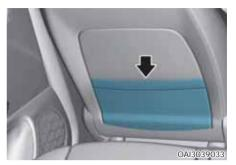
The seatback pocket is provided on the back of the driver's and/or front passenger's seatback.
