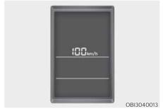
This message shows the speed of the vehicle (km/h, MPH).
