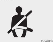
As a reminder to the front passenger, the front passenger's seat belt warning lights will illuminate for approximately 6 seconds each time you turn the ignition switch or Engine Start/Stop button ON regardless of belt fastening.
