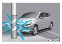
Air bags may not inflate if the vehicle collides with objects such as utility poles or trees, where the point of impact is concentrated and the collision energy is absorbed by the yehicle structure.
