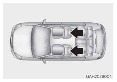
The driver's and front passenger's seats are equipped with a headrest for the occupant's safety and comfort.
