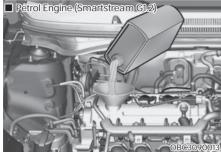
If the oil level is below L, add enough oil to bring the level to F (Full). Do not overfill.
