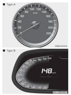
The speedometer indicates the speed of the vehicle and is calibrated in kilometers per hour (km/h).
