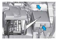
Inside the fuse/relay panel covers, you can find the fuse/relay label describing fuse/relay name and capacity.
